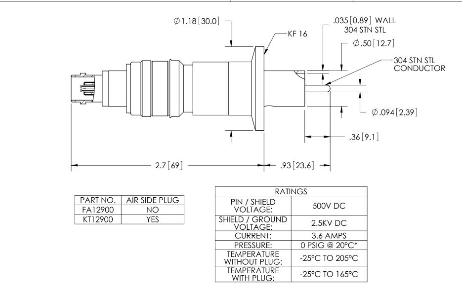
\*FOR INTERNAL PRESSURE 5 TO 100 PSIG AN OVERPRESSURE RING IS REQUIRED.
