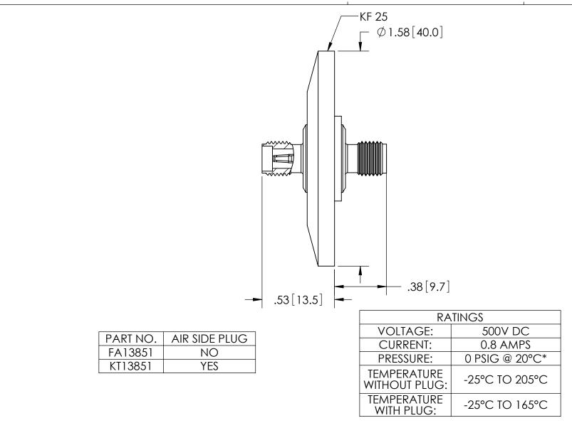
\*FOR INTERNAL PRESSURE 5 TO 100 PSIG AN OVERPRESSURE RING IS REQUIRED.
