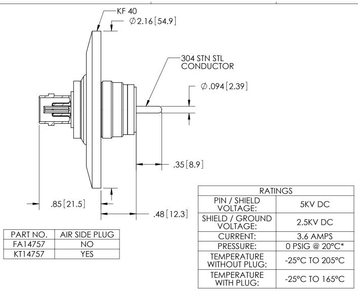
\*FOR INTERNAL PRESSURE 5 TO 100 PSIG AN OVERPRESSURE RING IS REQUIRED.
