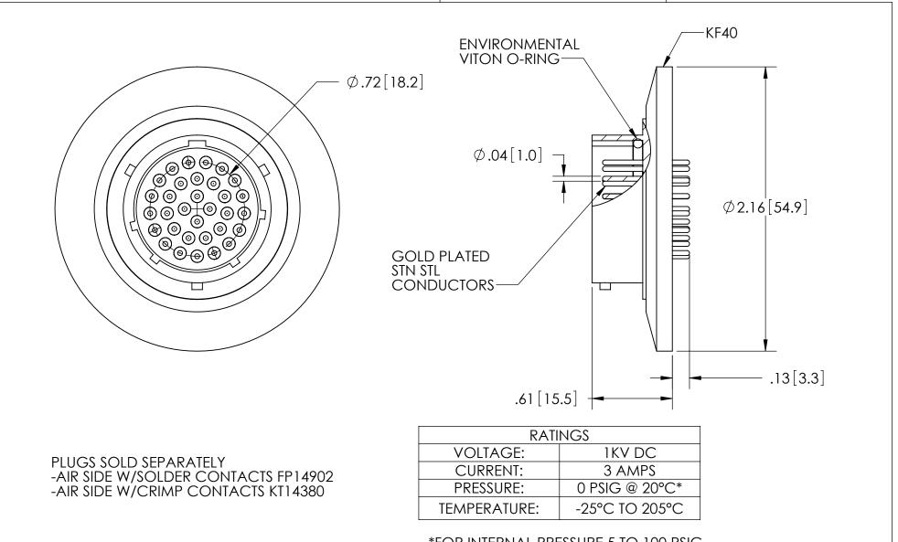
\*FOR INTERNAL PRESSURE 5 TO 100 PSIG AN OVERPRESSURE RING IS REQUIRED.
