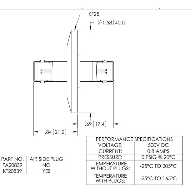
\*FOR INTERNAL PRESSURE 5 TO 100 PSIG AN OVERPRESSURE RING IS REQUIRED.
