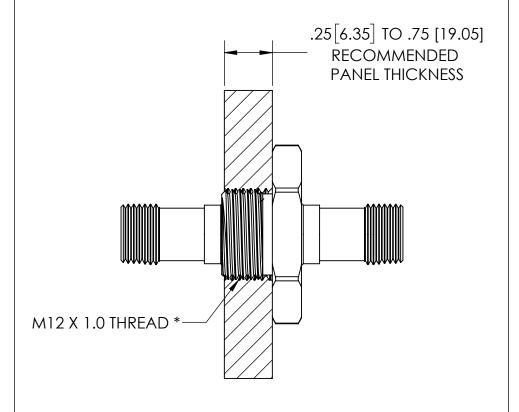
\* IF THREAD IS NOT TAPPED THROUGH, ITS DEPTH MUST BE AT LEAST .264[6.71]
