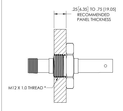
\* IF THREAD IS NOT TAPPED THROUGH, ITS DEPTH MUST BE AT LEAST .264[6.71]
