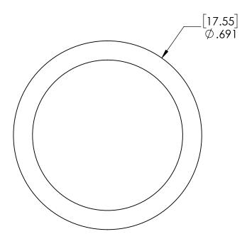
NOTES: THIS ACCESSORY O-RING IS FOR USE ON SST JAM NUT/ BASEPLATE OPTICAL FIBER FEEDTHROUGH ADAPTERS.
