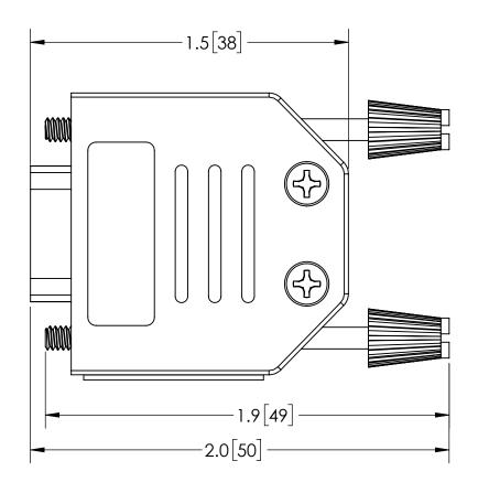
SPECIFICATIONS STEEL SHELL W/ TIN PLATING GLASS FILLED THERMOPLASTIC INSULATOR, RATED UL94V-0 BLACK PLASTIC HOOD - RATED UL94HB, HINGED W 4-40 THREADED THUMBSCREWS
