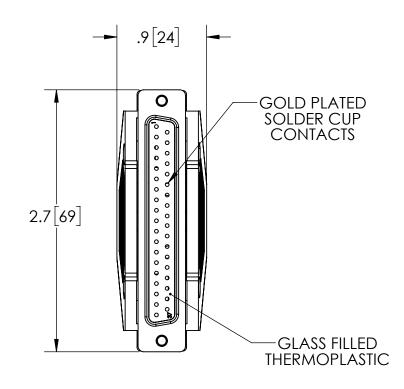
SPECIFICATIONS: RATED UL94V-0 STEEL SHELL W/ TIN PLATING THERMOPLASTIC INSULATOR GRAY PLASTIC HOOD
