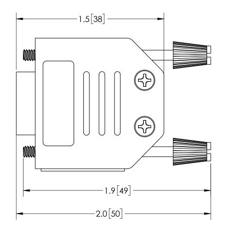
SPECIFICATIONS: STEEL SHELL W/NICKEL & TIN PLATING THERMOPLASTIC INSULATOR, RATED UL94V-0 BLACK PLASTIC HOOD- RATED UL94HB, HINGED W 4-40 THREADED THUMBSCREWS
