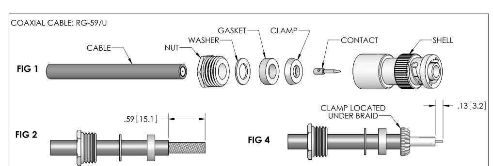
CUT CABLE END SQUARE. SLIDE NUT, WASHER, AND GASKET OVER CABLE. CUT JACKET TO DIMENSION SHOWN AND REMOVE.
