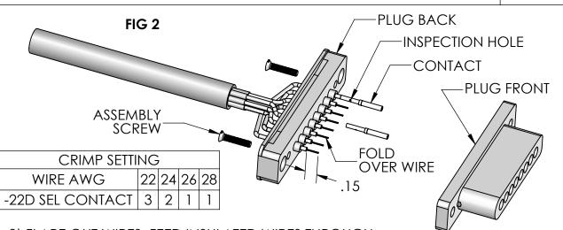
3) FLARE OUT WIRES, FEED INSULATED WIRES THROUGH PLUG BACK. STRIP INSULATION IF NOT DONE YET.
